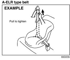
5) Try moving the child restraint system in all directions, to make sure it is securely installed. If you need to tighten the belt, pull more webbing toward the retractor.
